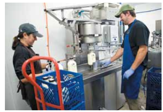
Left: Manning Hill Farm's stainless steel bottling machine fills milk into half-gallon reusable glass bottles.
