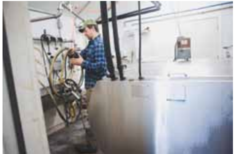
Left: Manning Hill Farm's stainless steel bottling machine fills milk into half-gallon reusable glass bottles.
